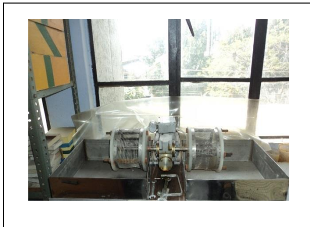
Figure 2.2: Slake Durability Test apparatus
