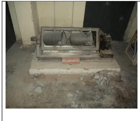
Figure 2.10: Deval's Test apparatus for attrition testing
