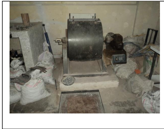
Figure 2.11: Los Angeles Test apparatus for attrition testing
