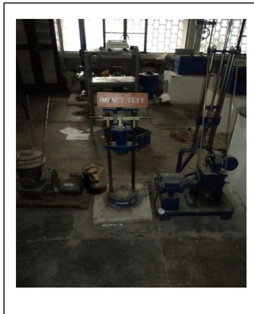
Figure 2.12: Aggregate Impact tester
