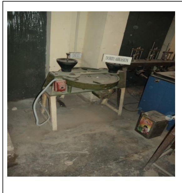
Figure 2.13 Dorry's Abrasion Test machine
